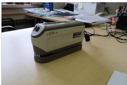
Sl. 23. Spektrofotometar ( SPECTROPHOTOMETER CM-2600d, Ver 1.42, (c) 2000-2013 KONICA MINOLTA, INC. )
